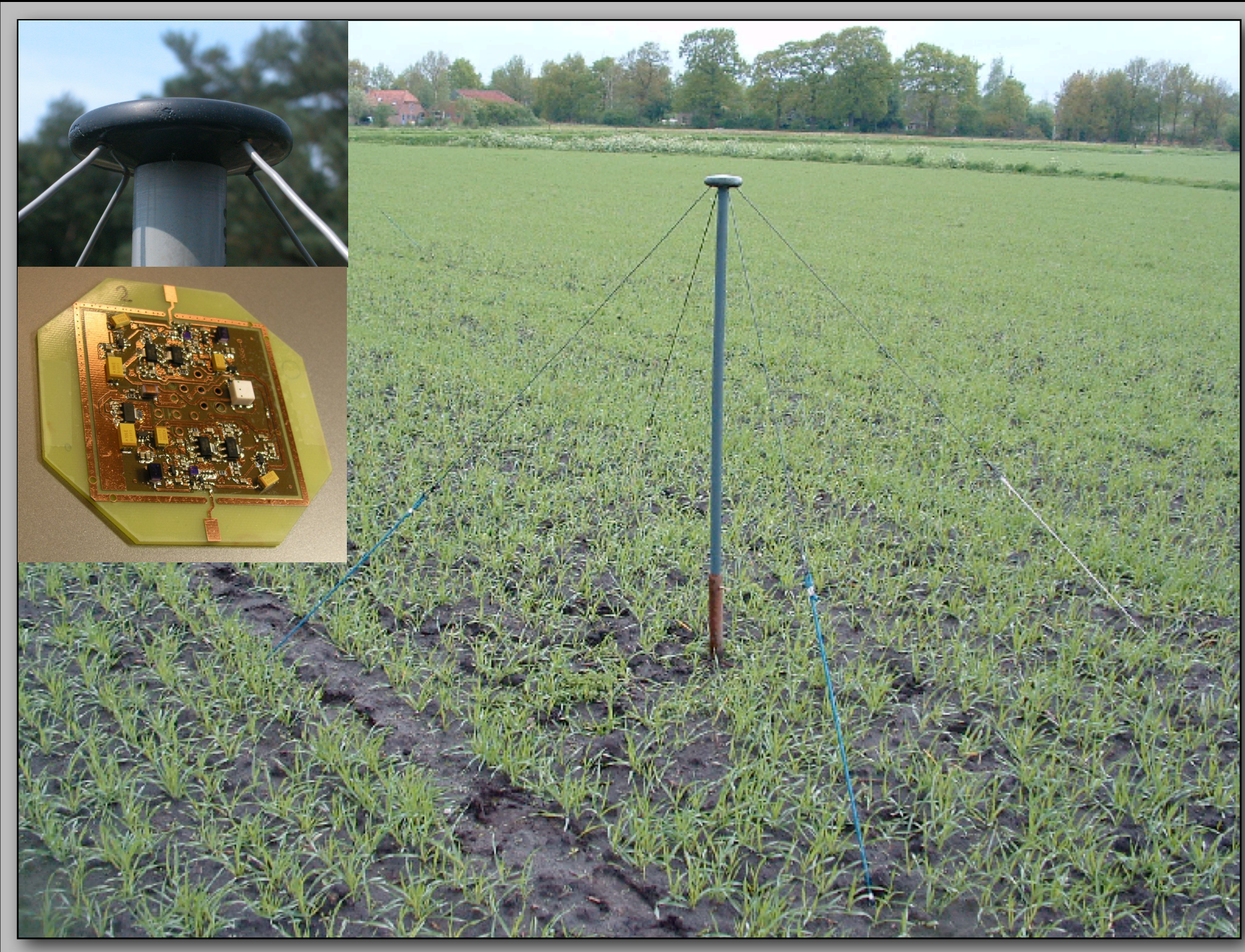
Low band antenna: 30 – 80 MHz 48/96 antennas per station
