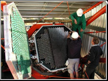
960 PMT pixels Angular pixel size: 0.16° Camera diameter:5° FoV (1.4 m)
